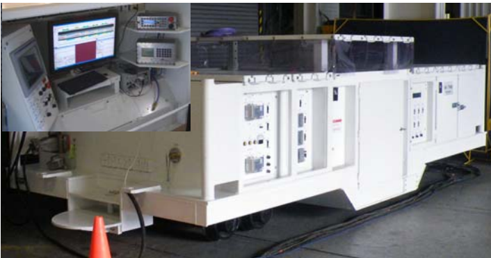
Figure 12. Operator car at the Pinnacle mine for control of the plow system.
