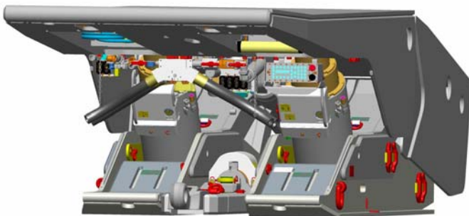
Figure 13. A face shield from the Pinnacle plow system – yield 5,162 kN
